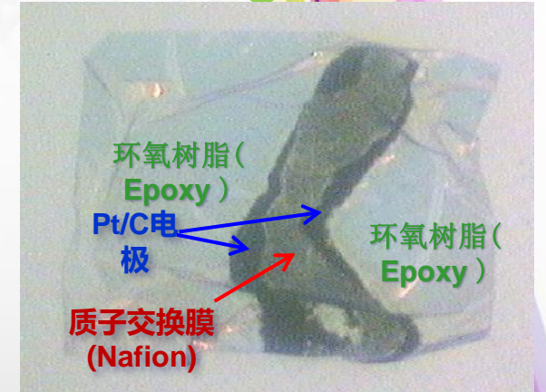
NEXSA optical image of ULAM-prepared MEA fuel cell
